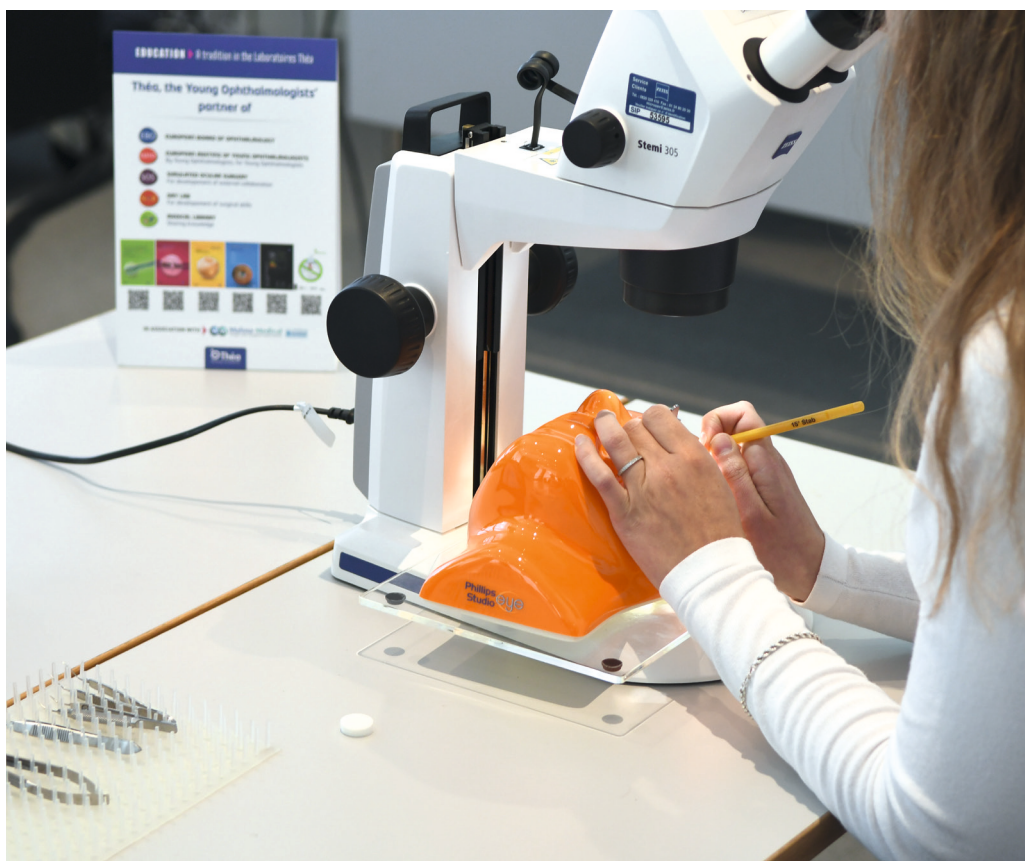
■ With training microscopes, it is possible to practice cataract and glaucoma surgery
