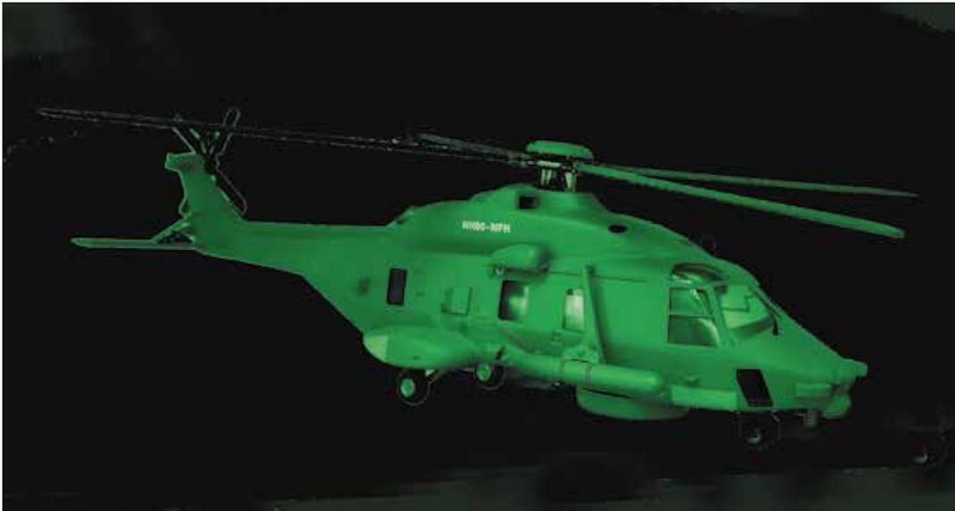
**Figure 6: Night vision goggles, where the visual field and objects appear green, is used by Norwegian military pilots on the new NH90 Helicopter. Photo: Atle Østern**
